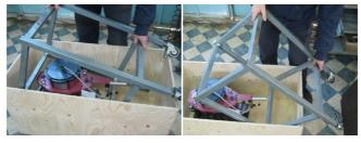
Unscrew the machine from the box and then hang the machine on the two hangers.
