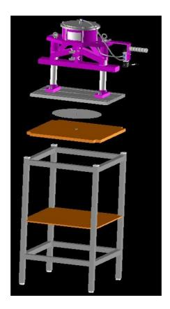
The machine should be able to rotate on the table and axis of the rotation should be the pin in the center of the wood. Note that the table should be ordered as accessory.
