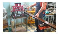
Only one profile is possible to be punched per stroke.
