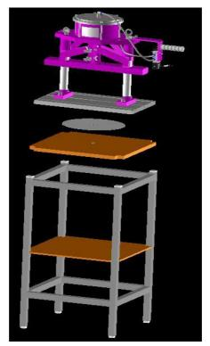
The machine should be able to rotate on the table and axis of the rotation should be a pin (Head of Allen Cap Screw M8) in the center of the wood. Note that the table should be ordered as accessory. The size on top must be 48cmx48cm otherwise so profiles will touch it.
