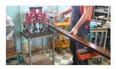
Only one profile is possible to be punched per stroke.
